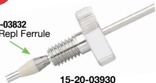
15-20-03930 EXP Nut & Ferrule Hand-tight to 8,700 PSI Wrench-tight to 20,000 PSI
