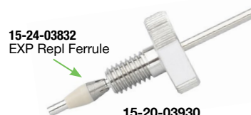
15-20-03930 EXP Nut & Ferrule Hand-tight to 8,700 PSI Wrench-tight to 20,000 PSI
